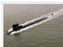
USS Richard B. Russell (SSN-687) in January 1984. Note the antenna buoy housing, or "bustle", behind her bow, which had been installed in August 1977.
